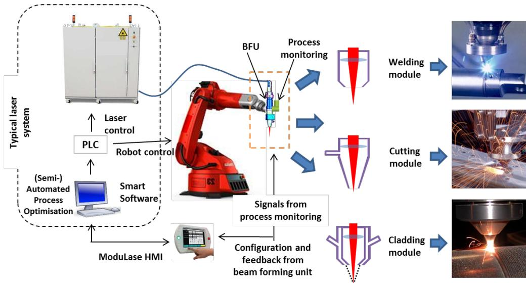
**Figure 1** Schematic overview of the ModuLase system, comprising a re-configurable process head (with BFU and modular end-effectors), process monitoring sensors, and a control system for adaptive process control and (semi) automated process optimisation.
